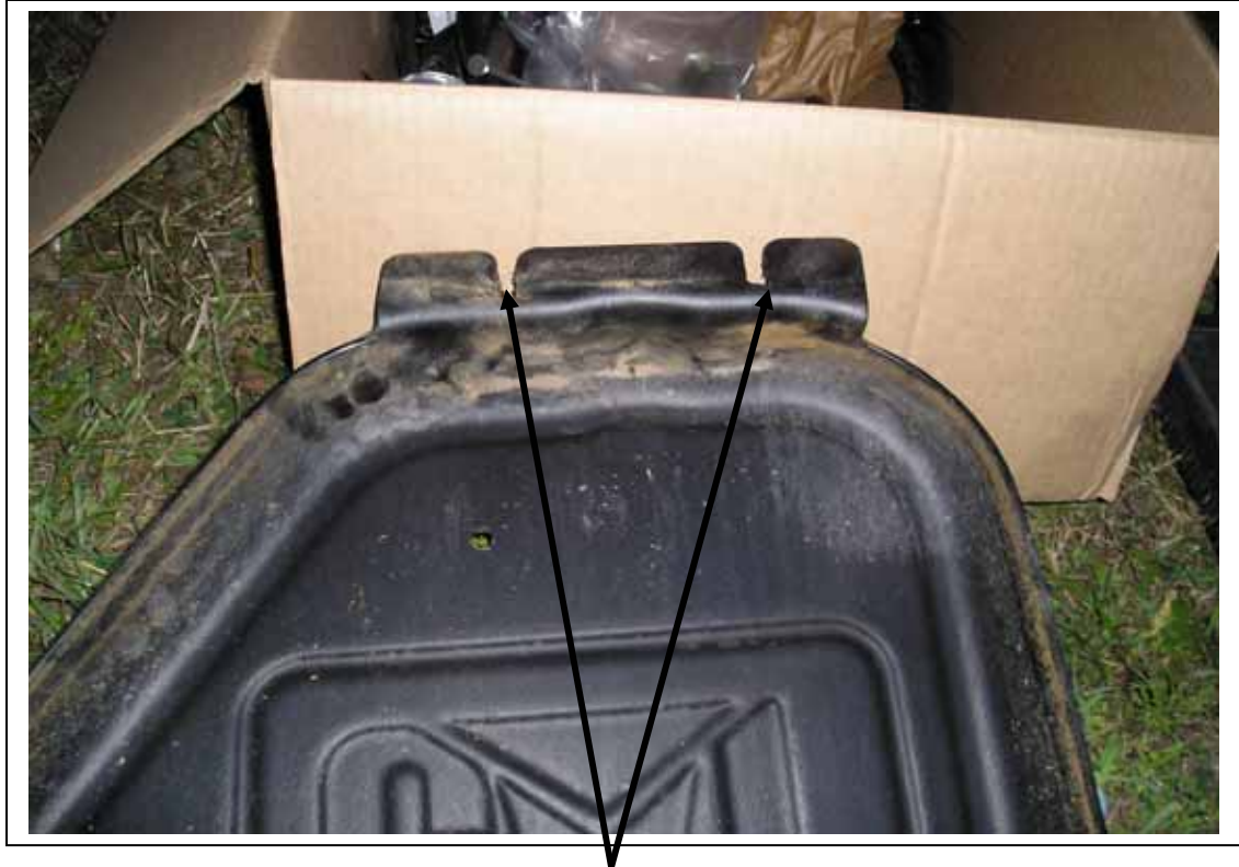
Make mounting slots for bottom of belt cover longer to give extra room for the add on pulley.
