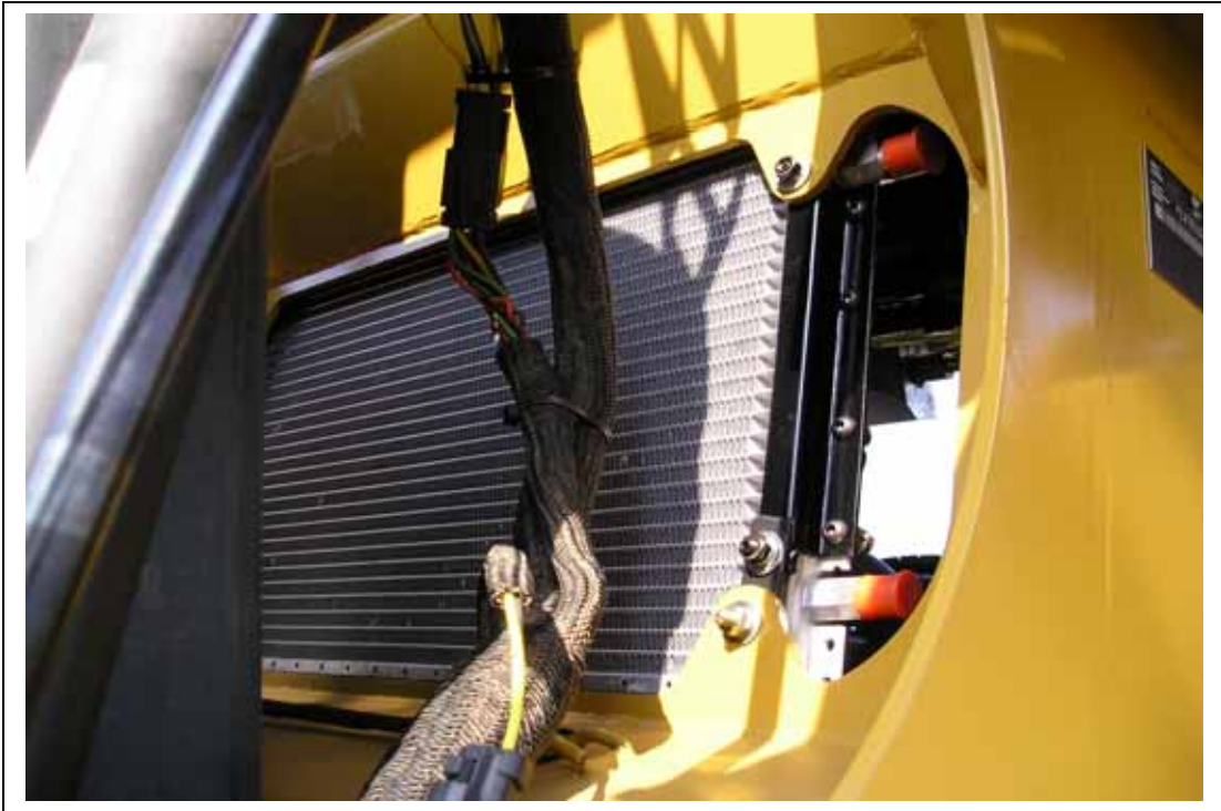
Fitting side of condenser as seen from fuel tank side.
