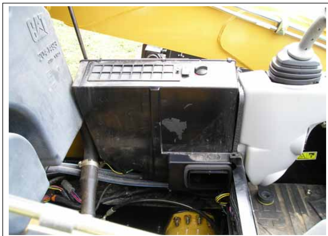
Heater box with cab up
