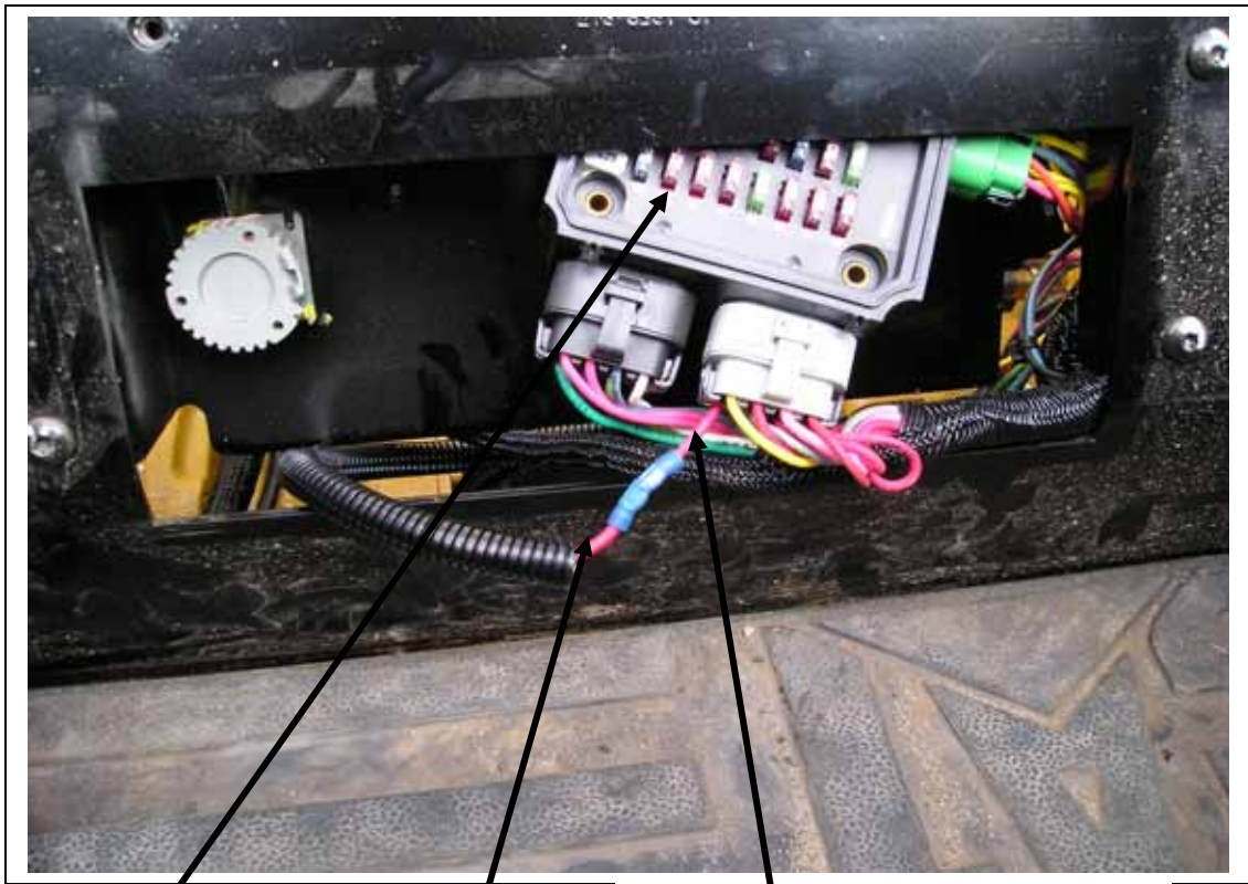
Wire # 125-A108 Cut wire out of bundle and splice on supplied 12g red wire.
