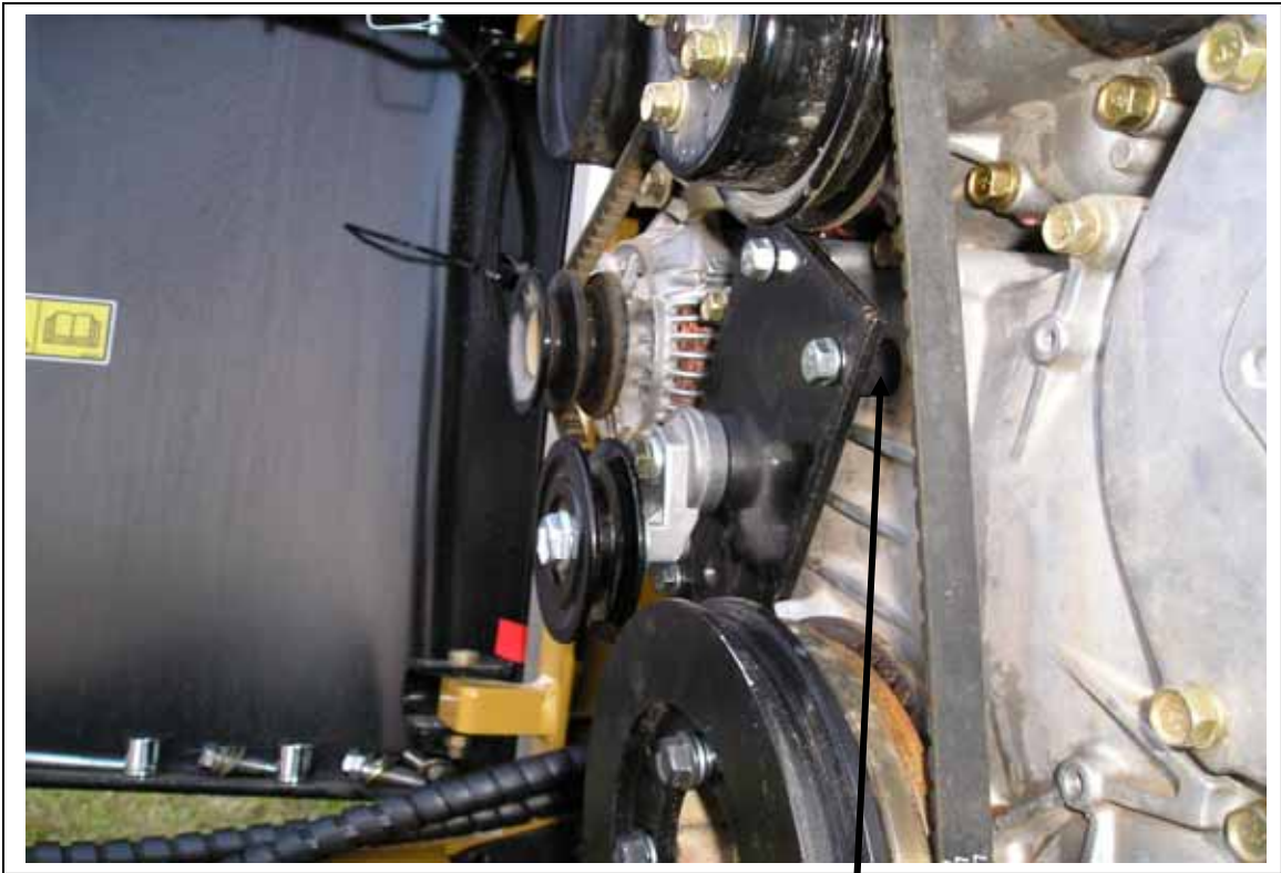
Standoff spacers for belt tensioner mount plate.
